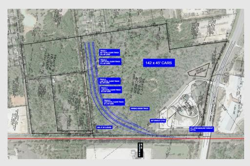
\*Rail design for conceptual use only. Alternate rail design has been approved by the railroad
